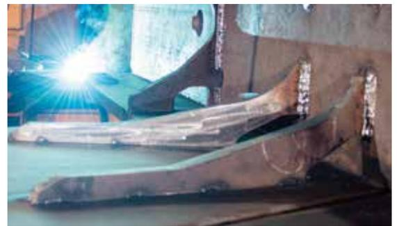
An unsurpassed weld surface, deep penetration: a crossbeam perfectly welded with just one layer.
