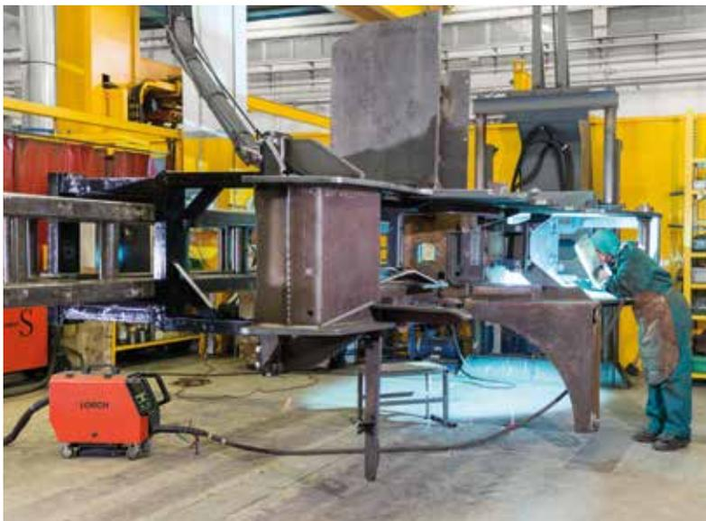
Ideal for large components: The Powermaster remote control allows welders to adjust their welding parameters directly on the torch.
