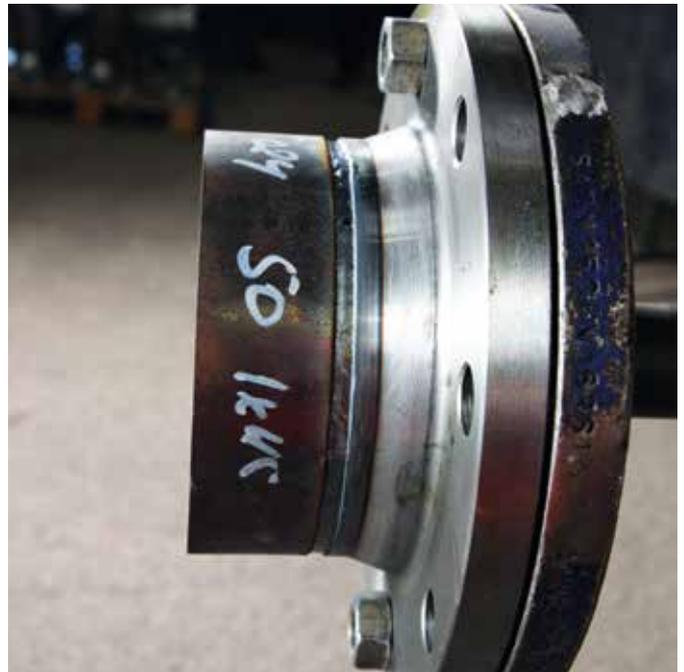
Lorch SpeedRoot: Spatter-free and requiring much less energy, SpeedRoot works three times faster than TIG welding even on an 8 mm gap during root welding.
