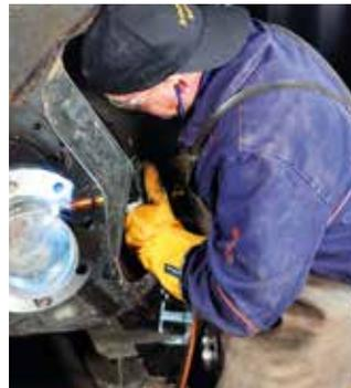
Applying Lorch's SpeedRoot process, Luis Braga uses an S-SpeedPulse system to weld the root layer of the pipe socket. The top layer is welded using Lorch's SpeedPulse process.
