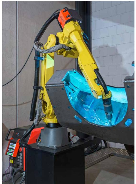
The seamless interplay of robot arm and positioner allows for welding in perfect downhand position
