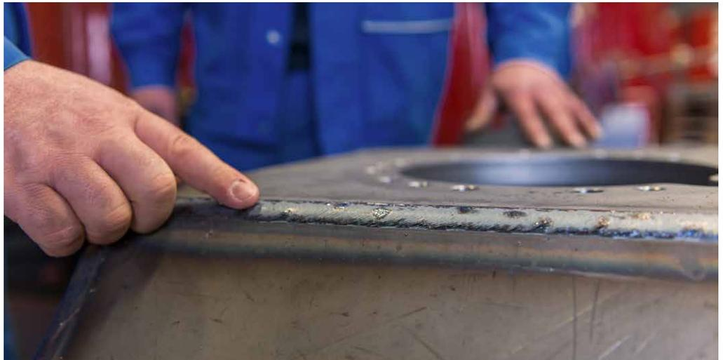
Top-grade surfaces, nearly spatter-free: Thanks to the use of robots, the need to rework each weld seam is reduced to a minimum
