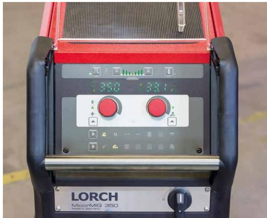
Everything in clear view: the control panel of the MicorMIG (here, the BasicPlus version). All three operating variants sport the same layout. Welding current and voltage are indicated on a digital display. End crater filling and multi-stage dynamic control can be selected directly via icons.
